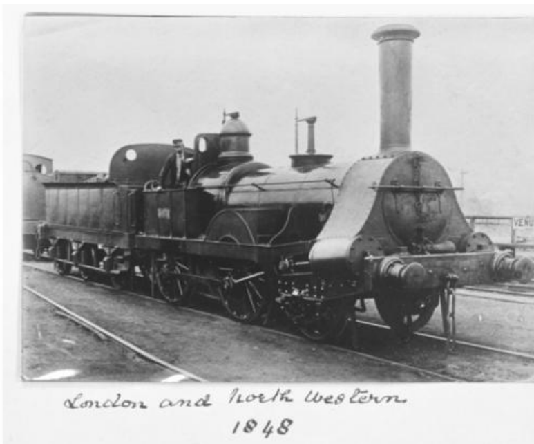
London & North Western Railway 2-4-0 locomotive, 1848. The railway operated between London & Glasgow (SSPL/Getty Images)
